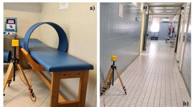
**Figure 5.** Picture of the measurements conducted near the magneto therapy device (panel a) and outside the room with the equipment (panel b).
