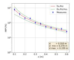
**Figure 1.** Interpolation of the weighted peak exposure index measured in the vicinity of an arc-welding device: d=31 cm is the nominal respect distance, d min =27 cm and d max = 33,9 cm are the values evaluated propagating the measurement uncertainty considering a coverage factor k=1.
